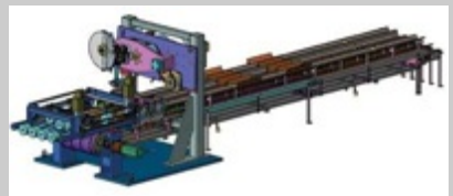
This rendering is of a Prolog LT log saw used to slice product at 250 cuts per minute for tissue and 125 for towel.
