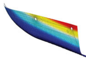
This COMSOL Multiphysics analysis of the viscoelastic behavior of a polymer resin airplane fairing strut during the cure cycle evaluates for final shape and residual stresses. The part undergoes various temperature/cure cycles to find the one with the best results.
