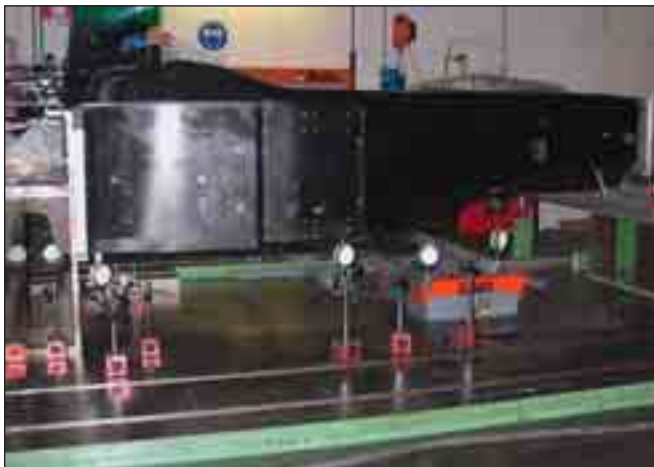
Figure 1. Chassis Flexural Stiffness test set-up.
