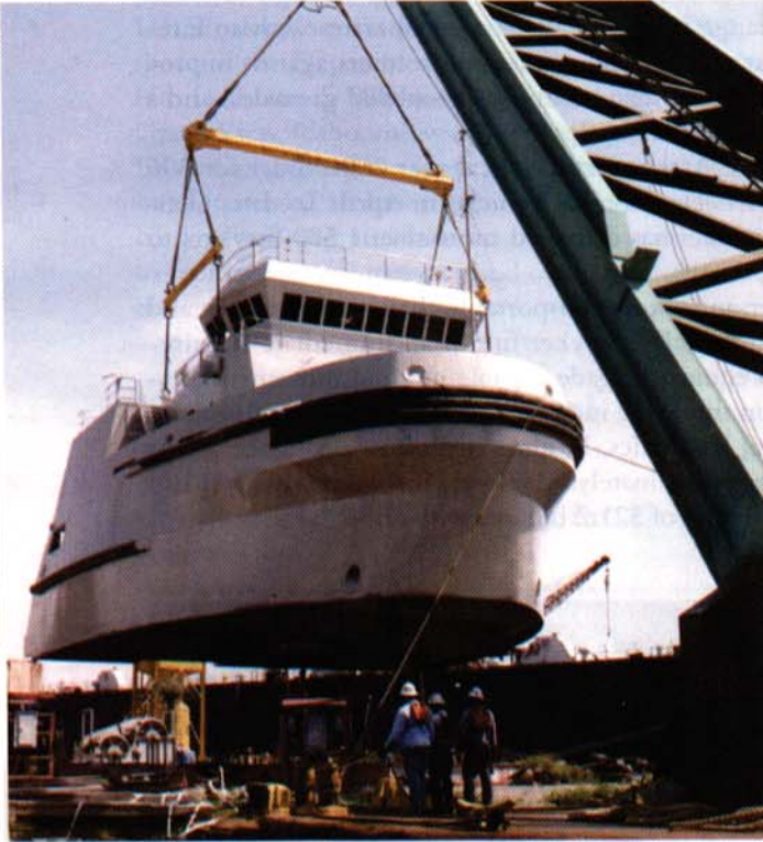
Ship parts need to be loaded precisely when they're being moved by crane. Software under development would make sure the parts are grabbed just right, so that they aren't damaged.
