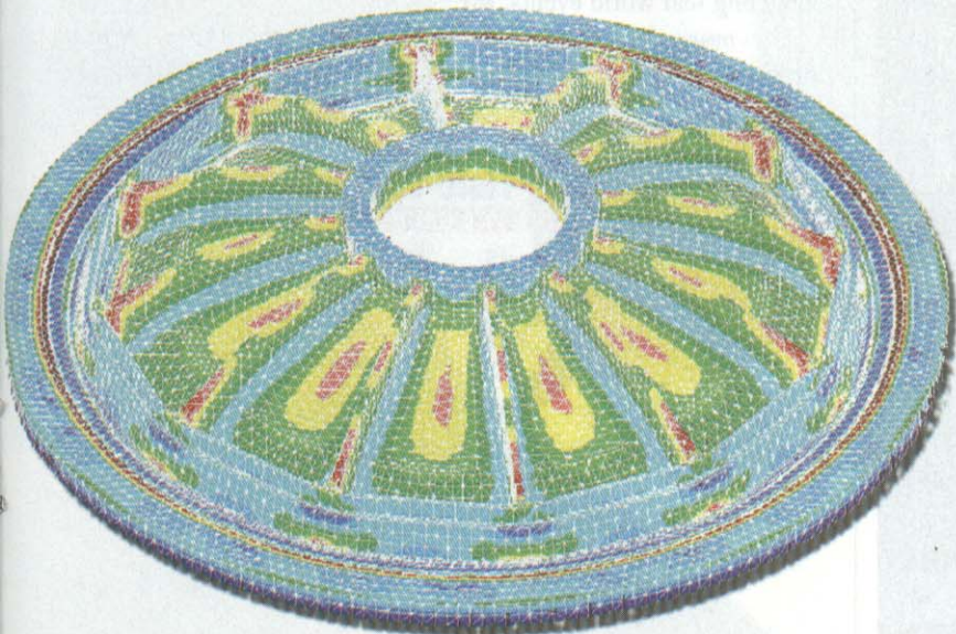
Nonlinear structural analysis on the rocket motor bulkhead for SpaceShipOne performed by SpaceDev, Inc. using NEiNastran FEA software.
