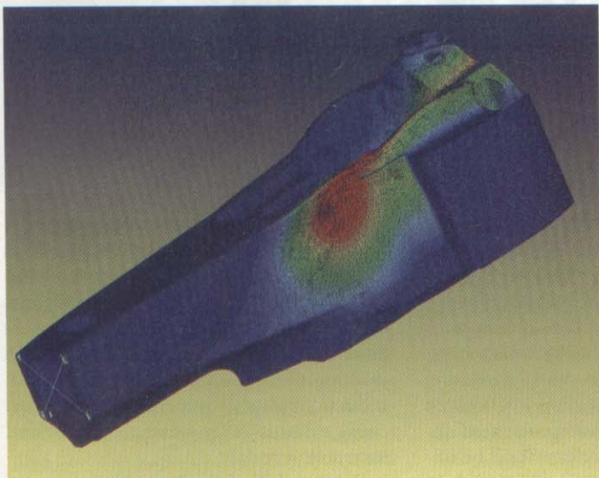
More than 15 impact tests, including side crash, were analyzed with NEiNastran.
