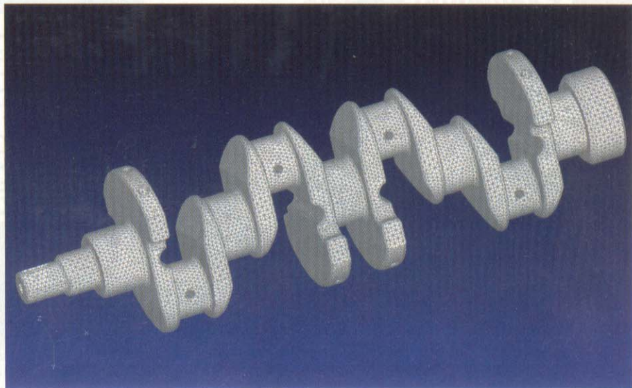
Noran Engineering's NEiWorks meshed this crankshaft model with TET10 elements for more than 1 million degrees of freedom. Its fine mesh density works well for complex shapes, offering accurate results.
