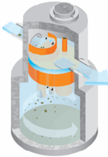
Stormceptor System with Fiberglass Plastic Insert
