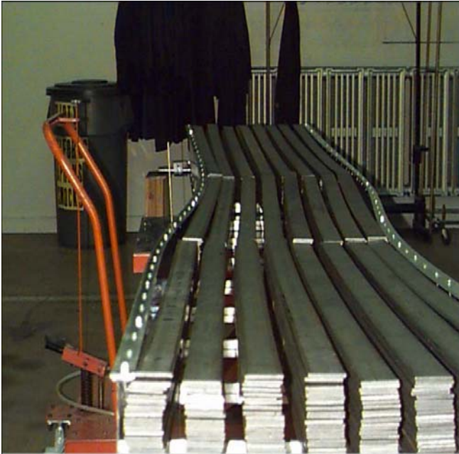
TEST – Gross Buckling of a Fully Loaded Ladder Tray
